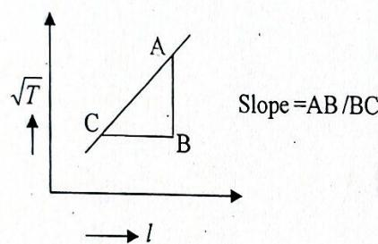
Formula : Frequency of AC source,  $n = \frac{1}{2\sqrt{m}} \left( \frac{\sqrt{T}}{l} \right) = \frac{1}{2\sqrt{m}} \times \text{Slope}$
