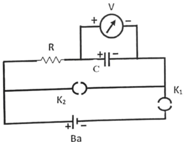
Where, V - Voltmeter (0-20 V DC), R - Resistor, C - Capacitor, K<sub>1</sub> & K<sub>2</sub> - Plug keys, Ba – Battery
